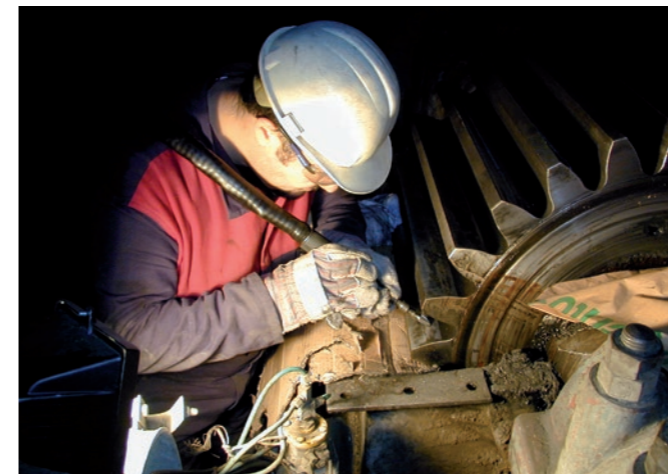
Grinding of pitting marks on the tooth flanks of a ball mill drive
