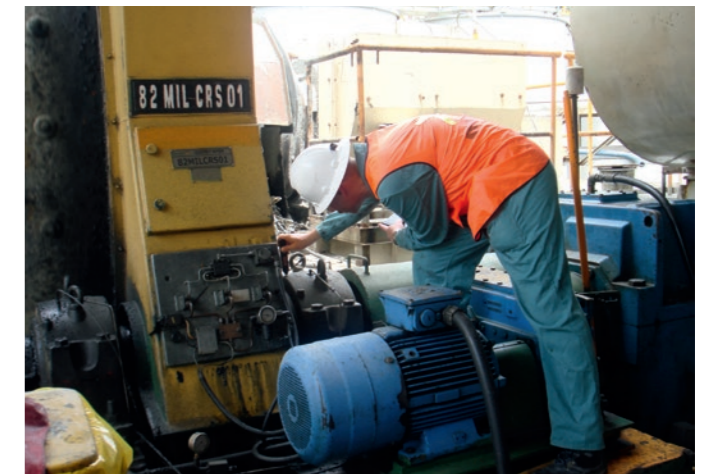
Vibration measurement at a ball mill drive
