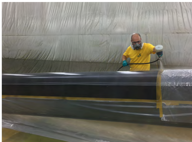
The surface coated with Berucoat AF 339 for telescoping is dry to the touch after one hour, can be subjected to load after 3 days, and after 7 days it has cured.
