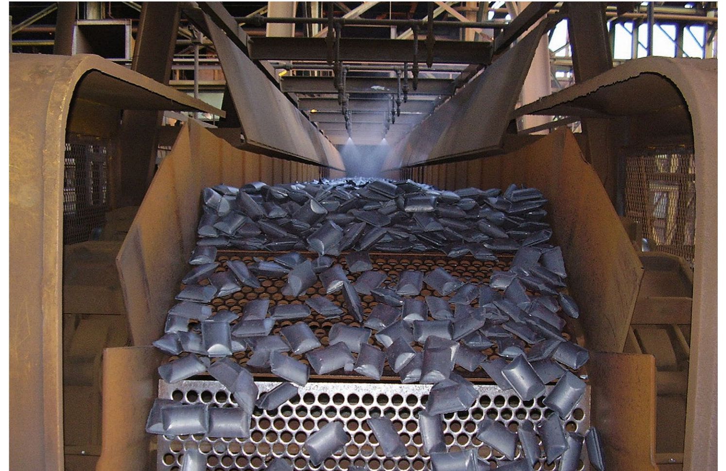
The hot briquetting represents a modern alternative to the blast furnace process
