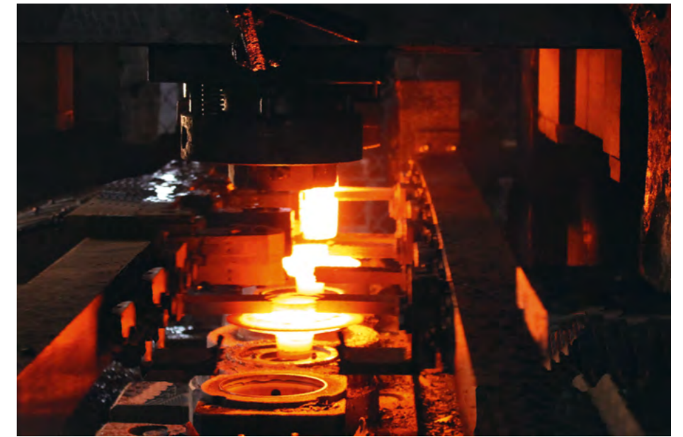
Berulit die spraying lubricants for optimized forging of automotive parts.
