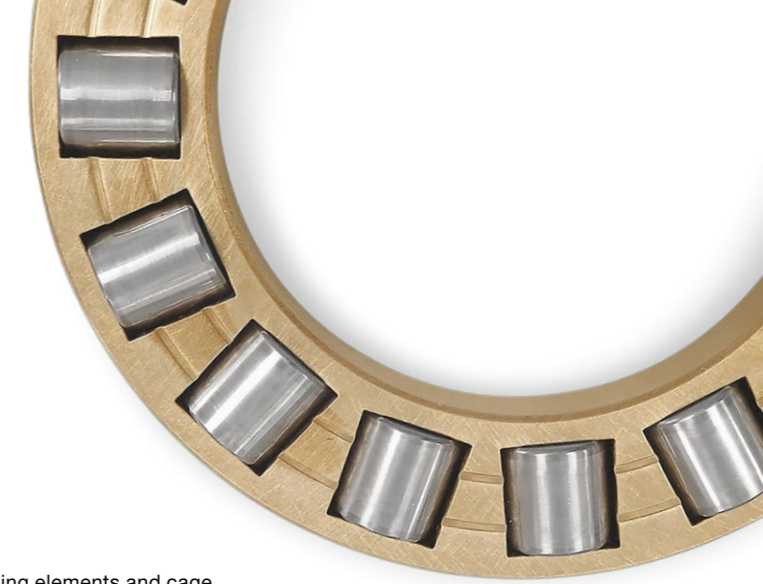
Rolling elements and cage of a FAG FE 8 bearing after the test run with Berusynth GPX gear oil
