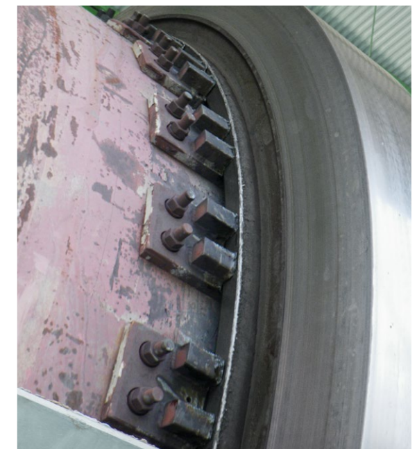
Well-lubricated tire at a rotary kiln
