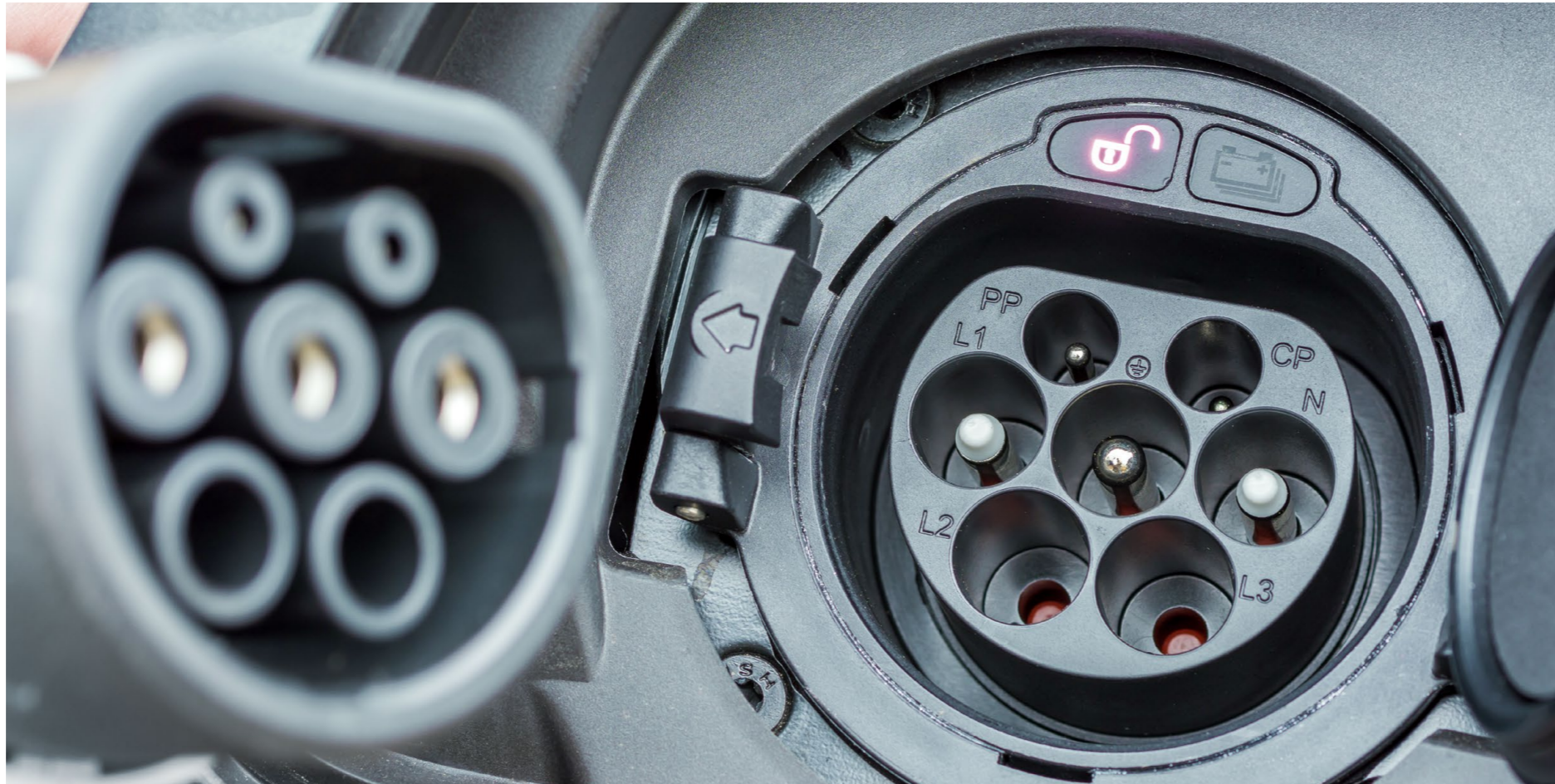
Risk of wear from high mechanical insertion and releasing forces
