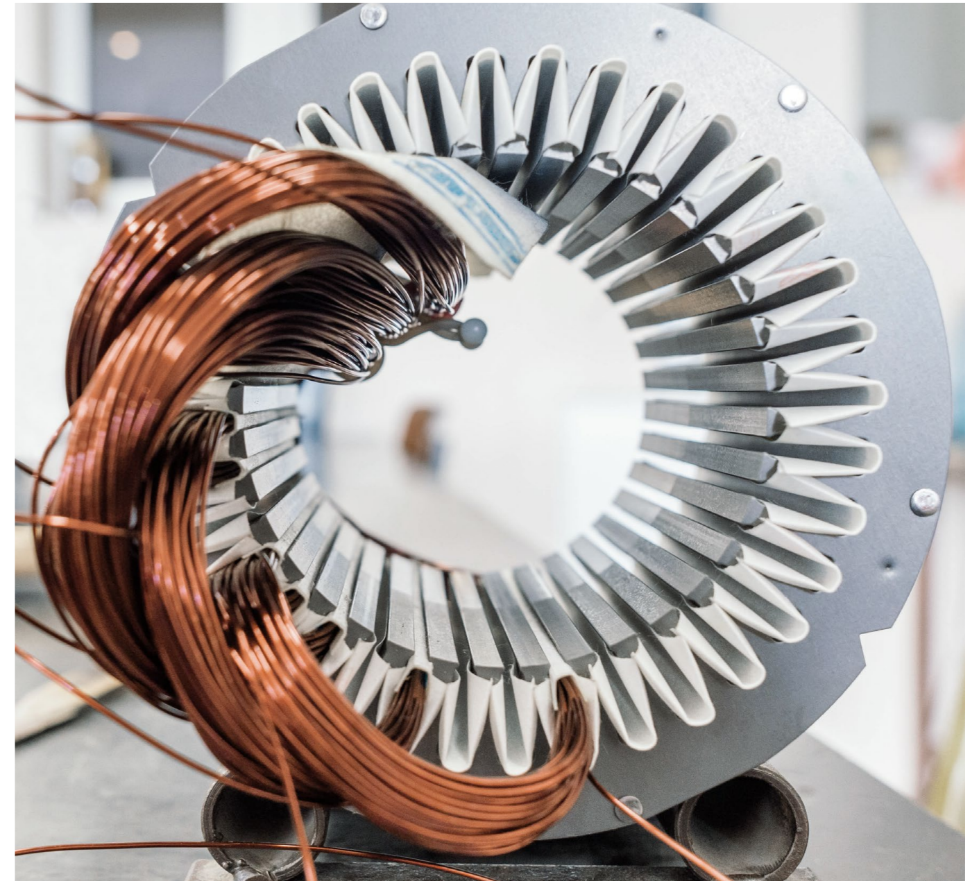
High-precision manufacturing with sharp punches is an essential part of electrical steel machining when it comes to building highly efficient electric motors
