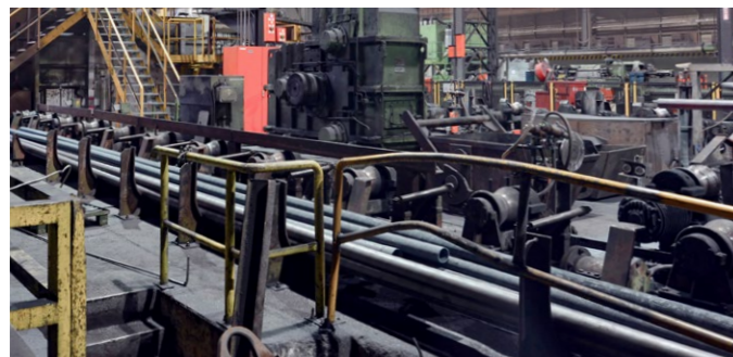
Tube mills require specialized lubricants to protect equipment in areas of high loads, water exposure, and high temperatures
